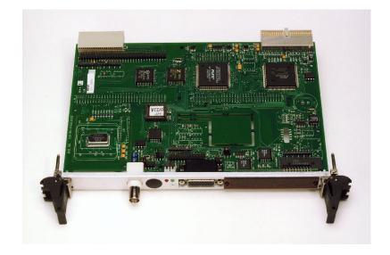
The CPCI-SyncClock32 from Brandywine Communications provides precision time with zero latency to the host computer over the CPCI bus. An on-board microprocessor automatically synchronizes the clock to reference signal inputs. The reference signal inputs can be 1 PPS, IRIG or NASA time codes and optionally, GPS or Have Quick. The clock can free run and be set by commands from the host over the CPCI bus.
