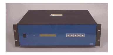
The Brandywine Communications M211 High Capacity Modular Timing System is designed for use in applications where a large number of reliable time/frequency outputs are required. These applications may include the display of time of day, synchronizing of computer systems or networks, telemetry and data acquisition system support or other diverse areas such as scientific experimentation and process control station synchronization.
